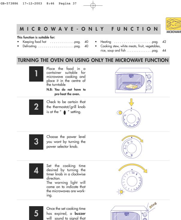
It is possible to interrupt the oven's operations at any time simply by turning the timer knob to its **STOP** setting. You may also change the cooking time (while the cooking itself is in progress) by turning that same knob back or forth.
