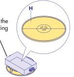
Functioning with thet urntable pin (D) Turntable operating Functioning without the turntable pin (D) Turntable not operating
